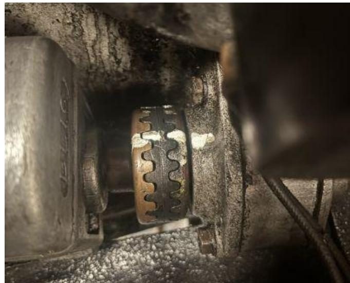
If you want to remove the magneto, then mark the alignment of the 2 brass couplings, and the intervening rubber vernier, so that the timing is not disturbed. I did this, but when I put it back in, the engine would not run at all. Eddie advised, and Ray Moses confirmed, that the Mag needed to be disconnected from the engine drive, and turned one complete turn, as there is a 2 to 1 reduction inside the Mag. This got it running again.
