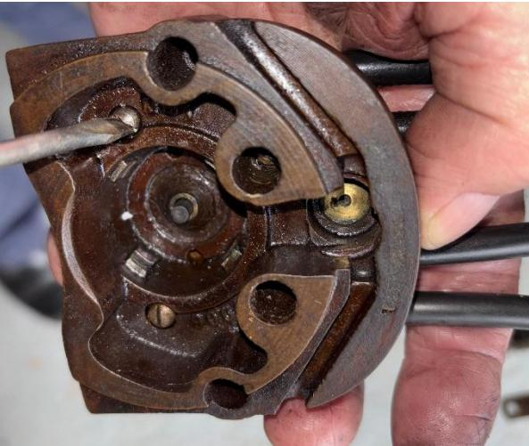
Step 7 Remove the contact breaker: on a BLIC (Birmingham Lighting and Ignition Company) Magneto, this is the lower black case at the rear, and slides off. This is necessary as the contacts are inaccessible whilst in the car. Clean the contacts with wet and dry paper, and then check the gap is about 15 thou.
