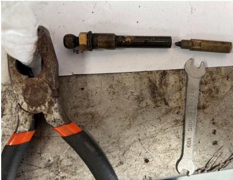
Use a 4BA spanner and pliers wrapped in padding to take the mixture jet off from its tube.
