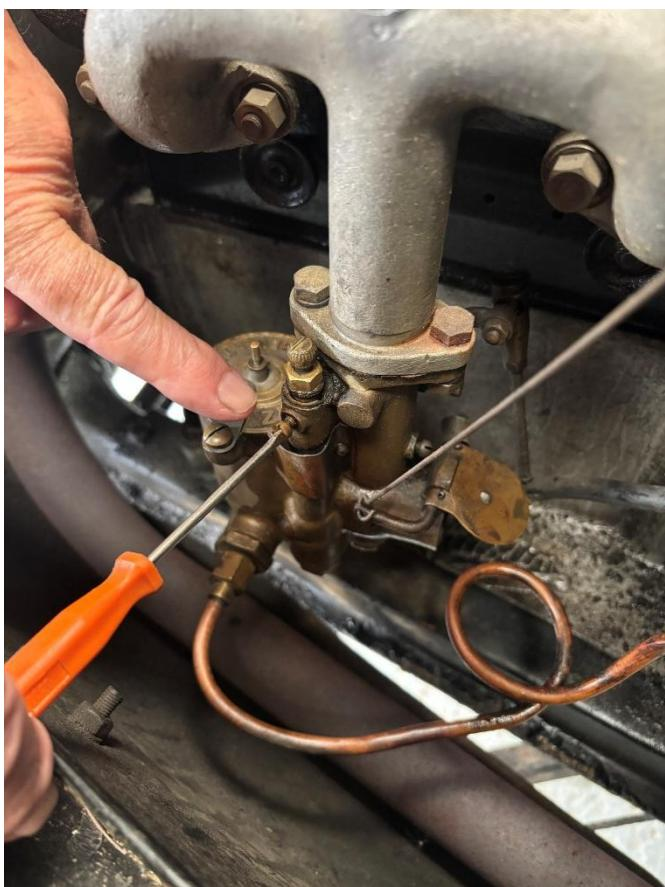
Step 3. Clean all three jets in Zenith carb. This should be done with air blasting, although I hear some use a very fine wire, such as from a wire brush.
